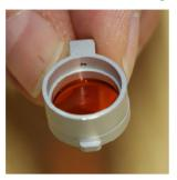
2. Place the orange filter on the **spot-on**®cordfree and screw in the grub screw using the Allen wrench.
