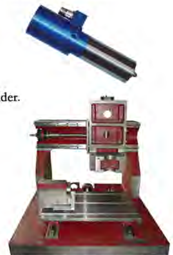
Cast structure with ribs
