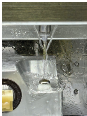
Optimum cooling with 3 special nozzles
